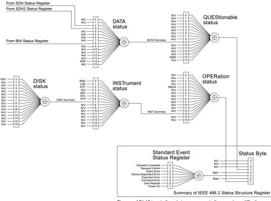
The use of Bit 15 is not allowed since some controllers may have difficulty reading a 16 bit integer. The value of this bit shall always be 0.
